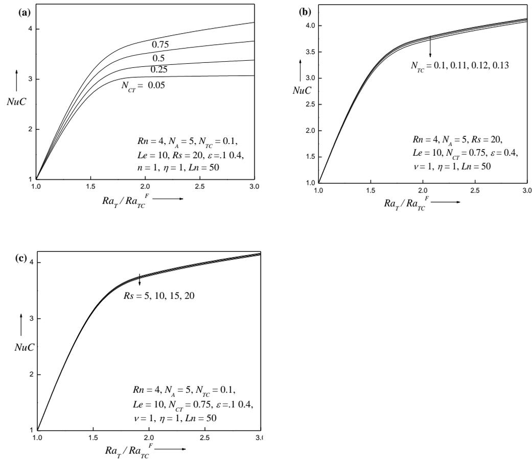
**Figure 5.** Variation of solute concentration Nusselt number  $NuC$  with critical Rayleigh Number for different values of (a) Soret parameter  $N_{CT}$ , (b) Dufour parameter  $N_{TC}$ , (c) Solutal Rayleigh number  $Rs$ .
