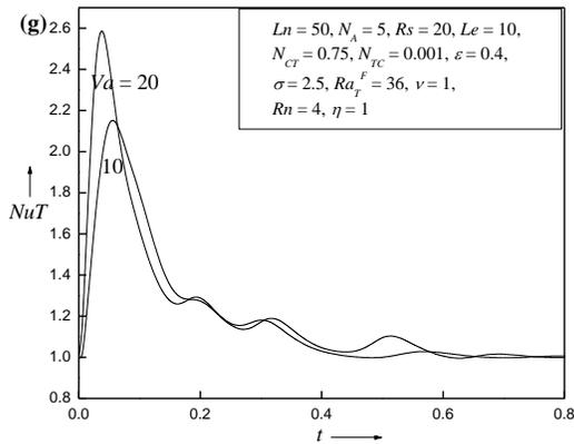
**Figure 6.** Transient Thermal Nusselt number  $NuT$  with time for different values of **(a)** Nanoparticle concentration Rayleigh number  $Rn$ , **(b)** Thermo-nanofluid Lewis number  $Ln$ , **(c)** Modified diffusivity ratio  $N_A$ , **(d)** Solutal Rayleigh number  $Rs$ , **(e)** Viscosity ratio  $\nu$ , **(f)** Conductivity ratio  $\eta$ , **(g)** Vadász number  $Va$ .
