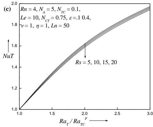
**Figure 3.** Variation of Thermal Nusselt number  $NuT$  with critical Rayleigh Number for different values of (a) Soret parameter  $N_{CT}$ , (b) Dufour parameter  $N_{TC}$ , (c) Solutal Rayleigh number  $Rs$ .
