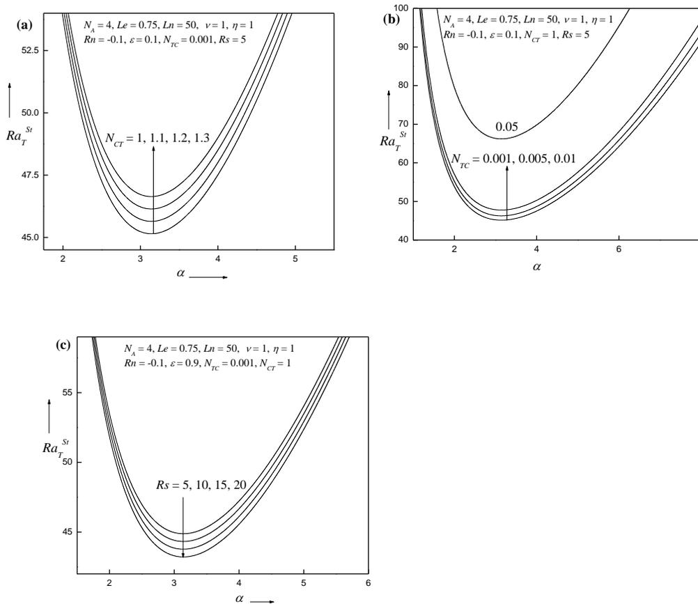
**Figure 1.** Neutral curves on stationary convection for different values of **(a)** Soret parameter  $N_{CT}$ , **(b)** Dufour parameter  $N_{TC}$ , **(c)** Solutal Rayleigh number  $Rs$ .
