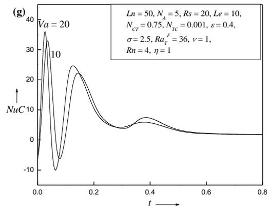
**Figure 8.** Transient solute concentration Nusselt number  $Nu_C$  with time for different values of **(a)** Nanoparticle concentration Rayleigh number  $Rn$ , **(b)** Thermo-nanofluid Lewis number  $Ln$ , **(c)** Modified diffusivity ratio  $N_A$ , **(d)** Solutal Rayleigh number  $Rs$ , **(e)** Viscosity ratio  $\nu$ , **(f)** Conductivity ratio  $\eta$ , **(g)** Vadász number  $Va$ .
