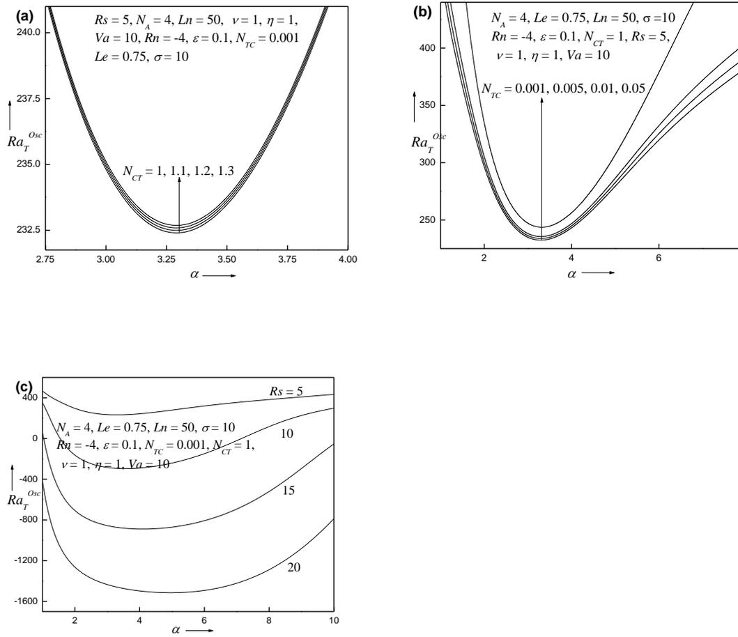
**Figure 2.** Neutral curves on oscillatory convection for different values of (a) Soret parameter  $N_{CT}$ , (b) Dufour parameter  $N_{TC}$ , (c) Solutal Rayleigh number  $Rs$ .
