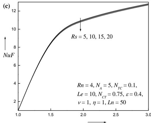
**Figure 4.** Variation of nanoparticle concentration Nusselt number  $NuF$  with critical Rayleigh Number for different values of (a) Soret parameter  $N_{CT}$ , (b) Dufour parameter  $N_{TC}$ , (c) Solutal Rayleigh number  $Rs$ .
